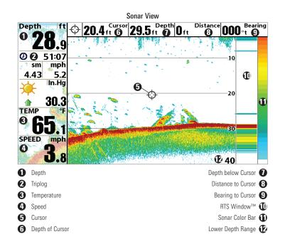
**NOTE:** If the Depth number is flashing, it means that the unit is having trouble locating the bottom. This usually happens if the water is too deep, the transducer is out of the water, the boat is moving too fast, or for any other reason that the unit can't accurately receive continuous data.
